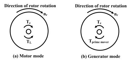
Figure 36.8: Direction of torques in rotating machines.
