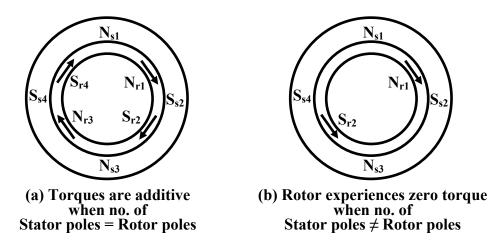
Figure 36.9: Direction of torques in rotating machines.
