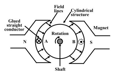
Figure 36.7: Single conductor rotating machine.
