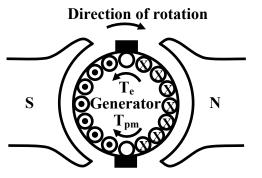
Figure 36.11: D.C Generator: principle of operation.
