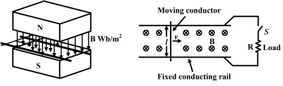
Figure 36.1: Elementary Generator Figure 36.2: Top view of figure 36.1
