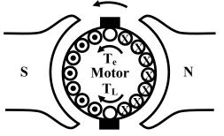
Figure 36.12: D.C motor: principle of operation.
