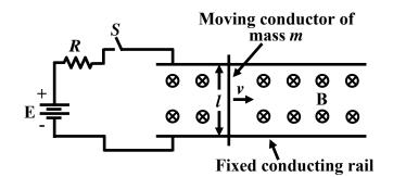
Figure 36.4: Top view during motor mode
